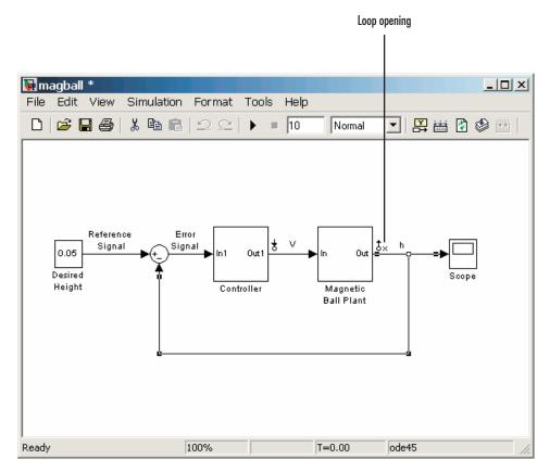
Create an I/O object based on the linearization annotations, create an operating point specification object for the model, and then find the operating point using findop.
